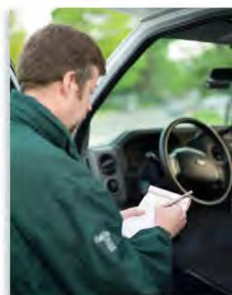
At the start of the day, operators perform a daily pre-trip inspection on every vehicle. The pre-trip inspection includes a 15-minute walk-around visual inspection and a check of the following:
