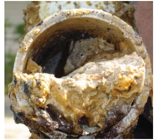
Grease clog inside a pipe.
