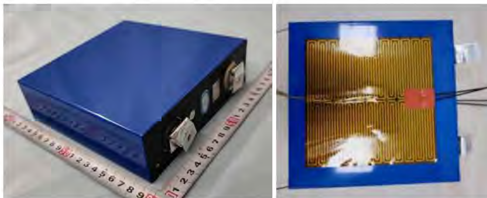
Figure 5 Individual cell tested to UL 9540A (left) and installed film strip heater (right).
