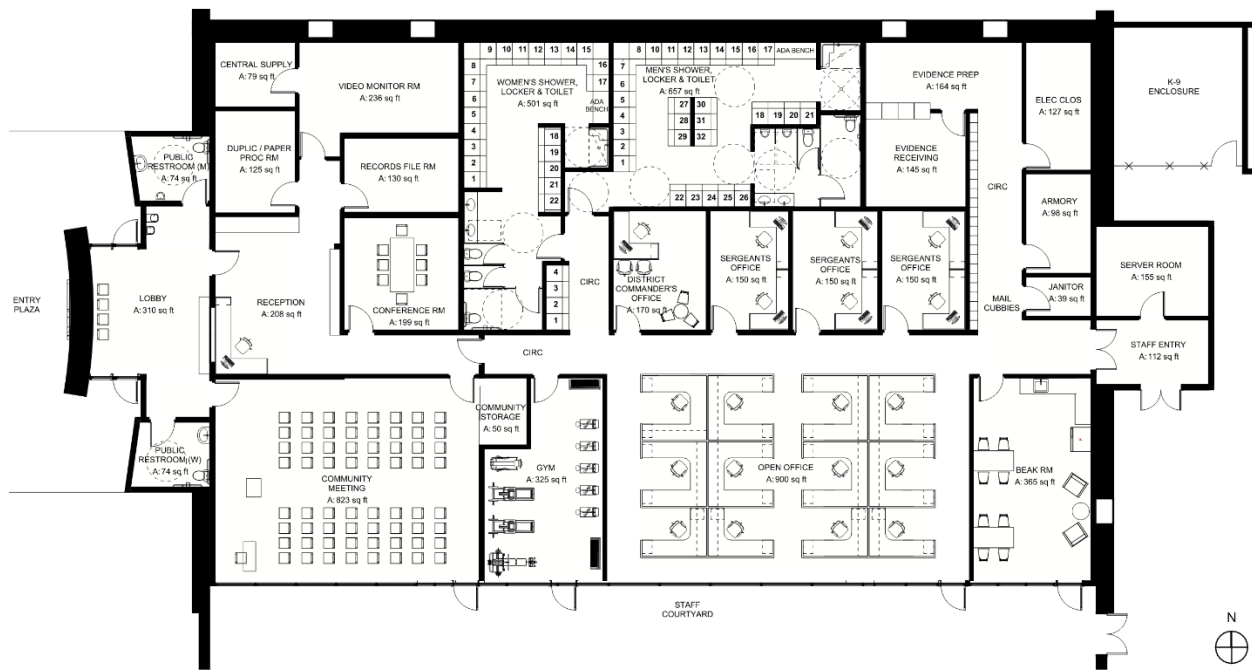
Figure 48 – Conceptual Floor Plan Option 1 with typical Male & Female locker rooms.
