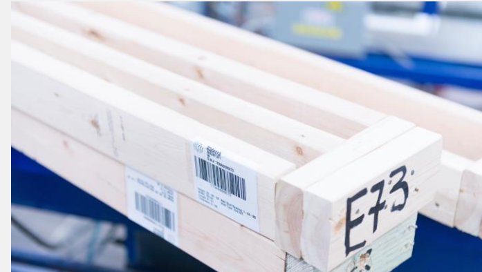
RFID tags are displayed to label and track components from design to jobsite.
