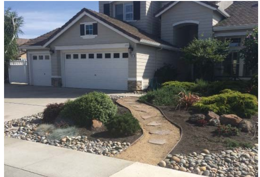
Example of a walkable permeable groundcover incorporating flagstone pavers and decomposed granite.
